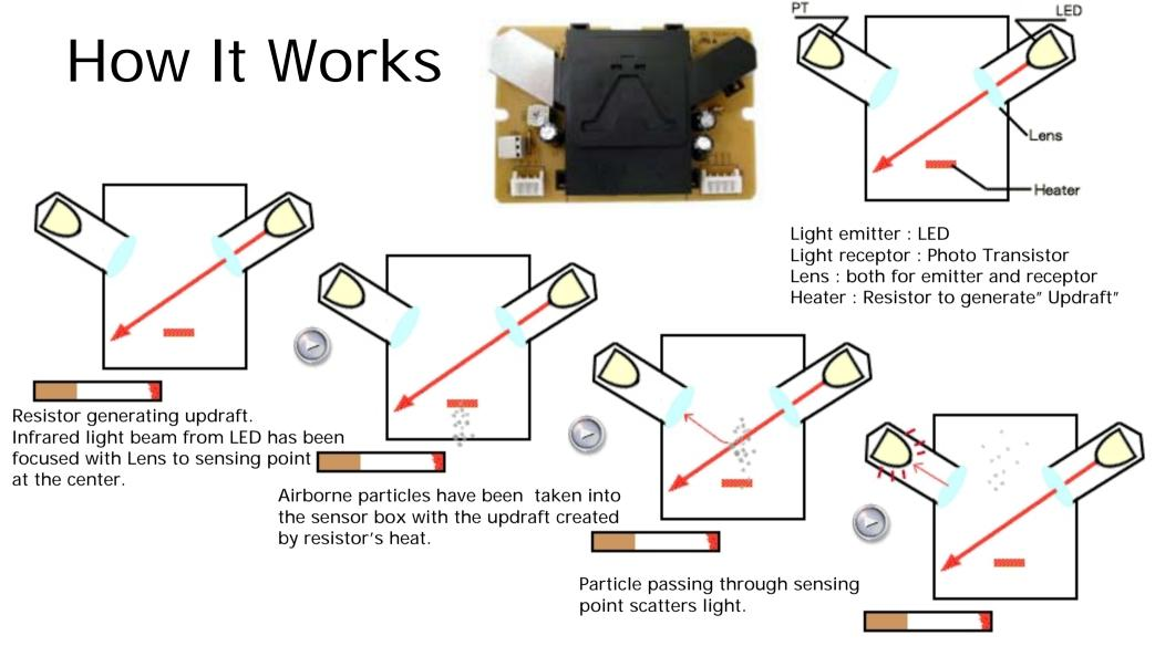
Receptor (Photo transistor) receive scatterec light through the lens and transformed into pulse signal. Pulse signal are to be converted into voltage output.
