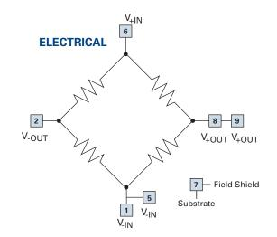
**Note:** Bridge output bond pads (V-out and V+out) correspond to topside pressure. For backside pressure, the bridge outputs are reversed.
