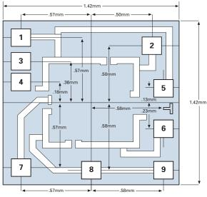
Bond Pad size = 0.15 mm x 0.15 mm Standard Bond Pad Metallization = Aluminum
