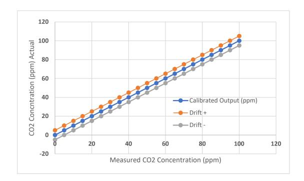
When the sensor leaves the factory, c = 0. However, over time and due to other environmental factors, the sensor can drift and gives rise to a non-zero offset value for c. The purpose of the auto-zero sequence is to re-baseline the sensor and reset c to a defined value.
