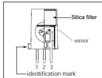
Fig 1c. Pin Layout
