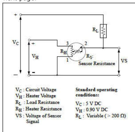
Fig 2. Standard circuit
