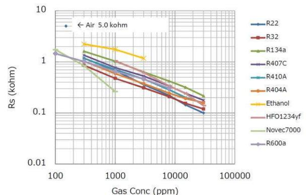
Fig3. Sensitivity characteristics
