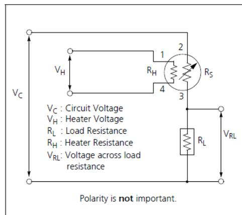
Fig 2. Standard circuit
