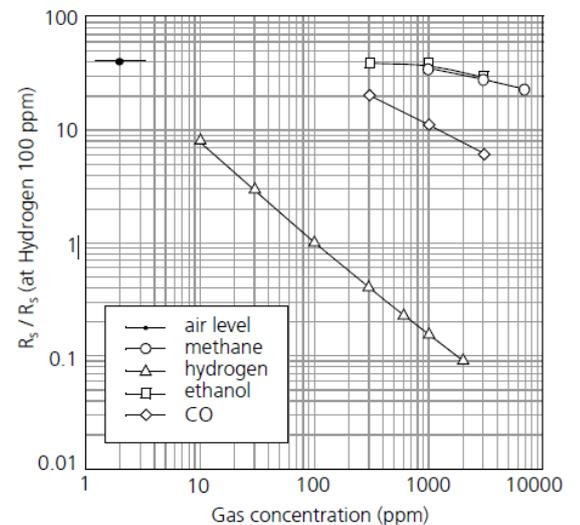
Fig 3. Sensitivity characteristics
