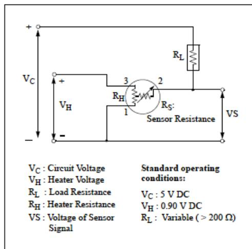
Fig 2. Standard circuit
