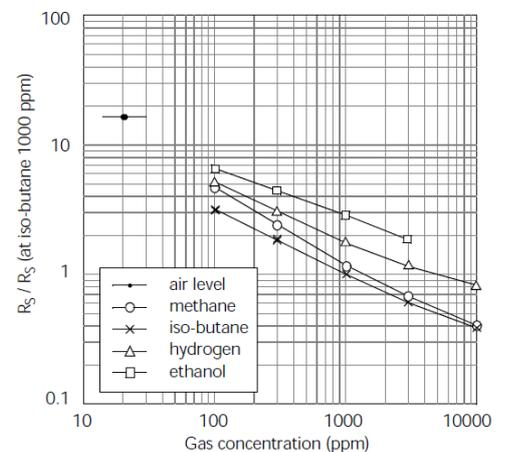
Fig3. Sensitivity characteristics
