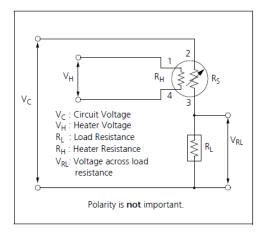
Fig 2. Standard circuit
