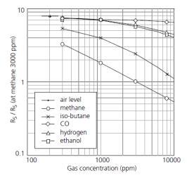
Fig3. Sensitivity characteristics
