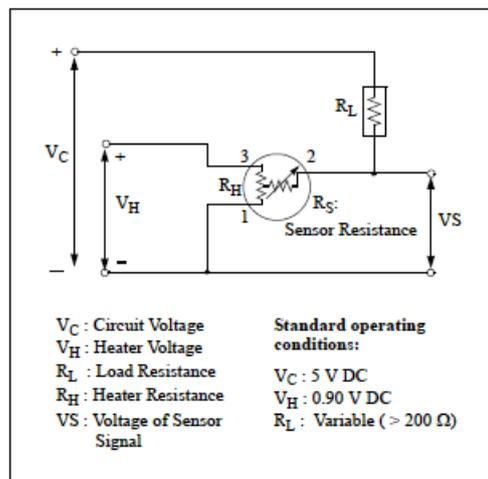
Fig 2. Standard circuit
