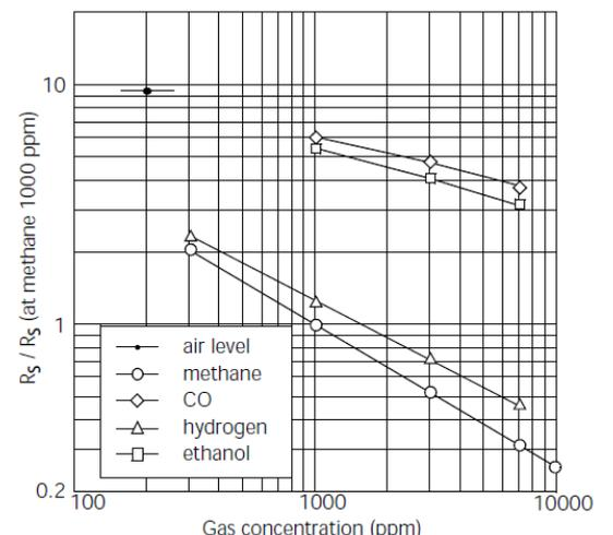
Fig3. Sensitivity characteristics
