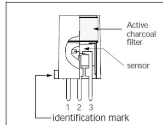
Fig 1c. Pin Layout
