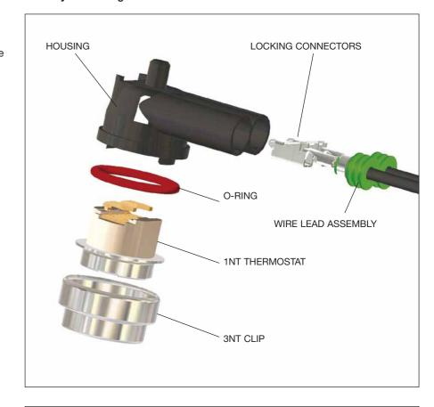
**Important Notice:** The 3NT is not hermetically sealed, and should not be submerged in liquid. For such applications, please contact Sensata Technologies for advice.
